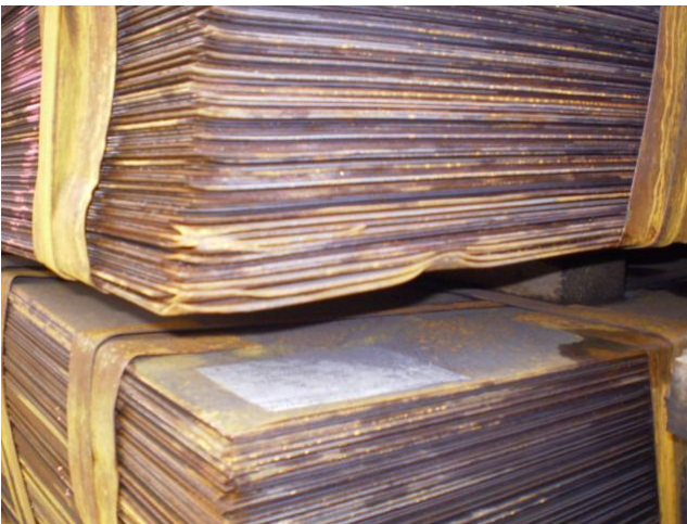
Pic. 6. Sheets with dented/buckled corners.
