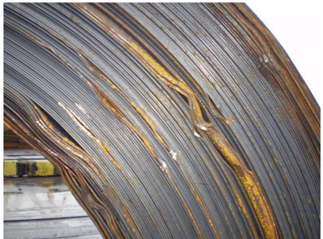
Pic. 7. Coil with buckled inner/outer windings
