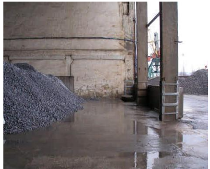
Pic. 3. Cargo of ferrosilicon in wet condition. View 2. As it is apparent from photos, despite the fact, that cargo is stored in shed warehouse, part of the cargo is located in puddle of rain water, cargo is partly wet.
