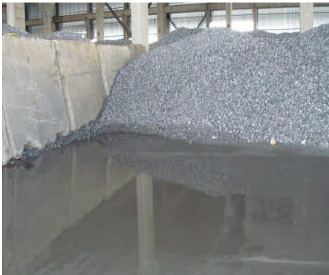
Pic. 2. Cargo of ferrosilicon in wet condition. View 1
