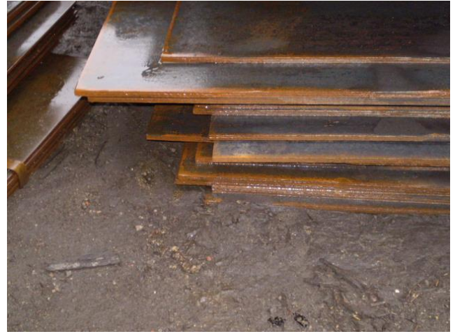
Pic. 5. Cargo partly rust stained.
