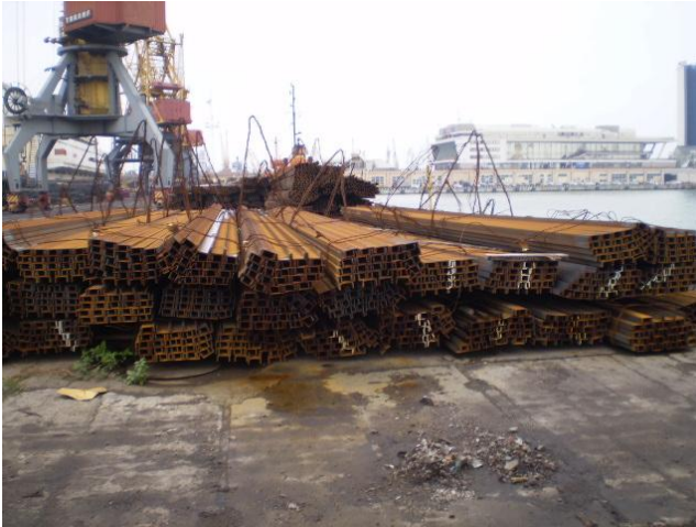
Pic.4. Cargo stored at open yard unprotected from elements.
