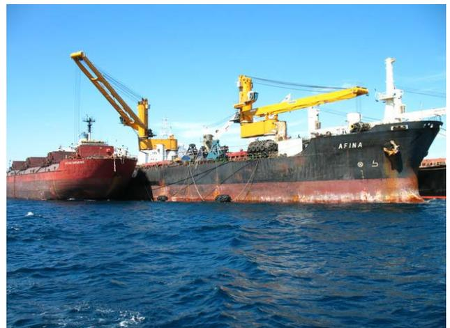
In this particular example the special vessel is loading the cargo from barge berthed starboard side alongside and discharging cargo to the vessel berthed portside alongside.
