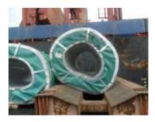
Type of steel mostly imported is galvanized and painted sheet steel in coils, to be used mostly for profiles for roofs, fences and other objects required long term physical protection. Oval and edge damaged coils as a result of too many tiers of coils and over pressure during carriage in such stowage on board
