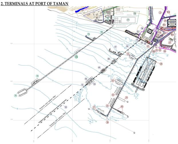
All Taman port terminals are located in open sea with connection to the shore. Therefore, safety of berthing is highly depending over weather conditions, wind and swell. Staying alongside the berths of this port can be highly dangerous for the vessel. There were several cases with damages to fenders of the berths due to delayed issuance of weather warnings by port authorities to the vessels and tugs, while the Masters of vessel were noticing quick deterioration of weather.
